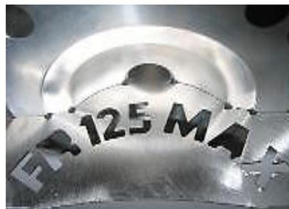
Height [H] of combustion chamber insert has to be 28,80 mm +/- 0,2 mm.
