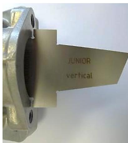
The template has to be moved in horizontal and vertical Position as far as Possible into the exhaust port.
