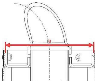
The Exhaust must be installed firmly to the chassis using a rigid mount/s.
