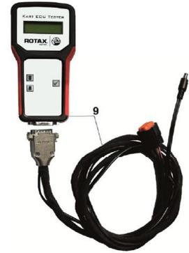
The ECU must be checked with the ECU tester (Rotax 276230) according to following procedure.
