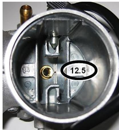
Angular bore of carburettor insert
