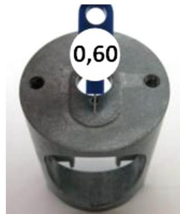
Vertical bore of carburettor insert
