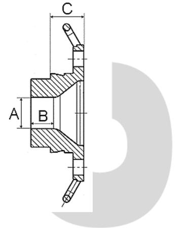
The internal profile of the exhaust socket has to be checked with the template, Rotax 277 405.
