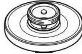
The two vent fittings must be connected with the original air vent hose min 155 mm (Rotax 260260). The location of the opening has to be placed at the rear side of the carburettor
