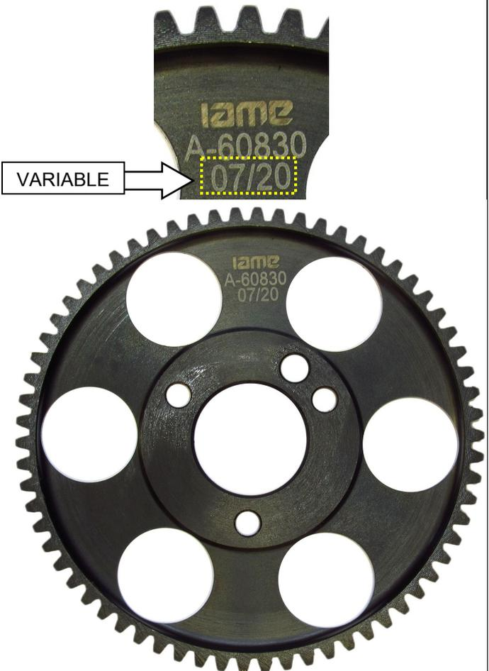
CRANKSHAFT AND HIS COMPONENTS IDENTIFICATION MARKING
