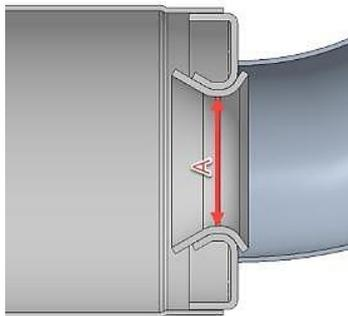
A steel ball with 28.0mm diameter **must not** pass through Section "A" and
