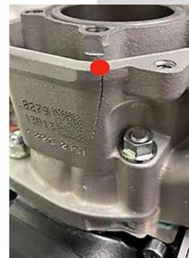
Example 2, Exhaust valve flange area repair. Only allowed on cylinder ID codes 223933 and 613933.
