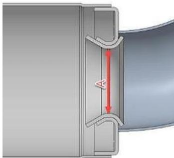
A steel ball with a 28.0mm diameter **must not** pass through Section "A" and
