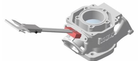
Measure the distance from the end of the gauge to the stopper surface of the cylinder.
