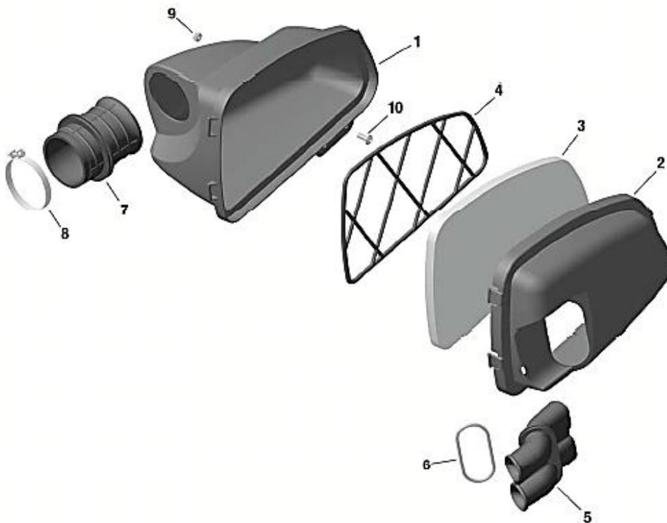
At intake silencer cover (Pos 2, Rotax 225022), it is mandatory to fit the O-ring (Pos 6) on the intake silencer tube (Pos 5). Intake silencer tube (Pos 5) and carburettor socket (Pos 7) are marked with the wording "ROTAX".
