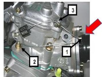
The 2 x distance plates must be engraved “ ROTAX “ (as per the drawing below)
