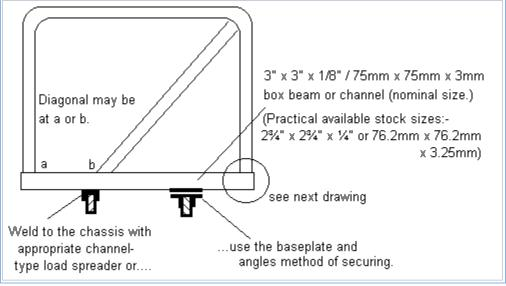
Where the main hoop connects to the chassis, a reinforcement made of an inverted 'U' channel must be locally welded between the tube and the chassis. There must be no gaps between the channel and the chassis and the 'U' channel must be 3" deep, 6 mm thick and
