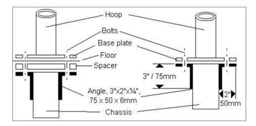
Above left: - Bolting through a floor. The angle iron is welded to the chassis and a spacer / packing piece will almost certainly be needed to fill the gap.
