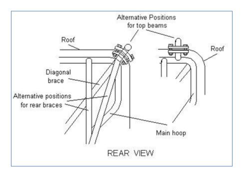
Since many vehicles are now being equipped with external cages the fitment of rear braces on the interior is not possible. As a stop gap solution for such cages the rear braces must be done externally between the top corner main hoop and the bottom rear corner of the end
