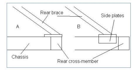
"A" shows the rear brace on top of the rear cross-member. No chassis side plates can be fitted, so a flat plate over the rear cross-member and overlapping on to the chassis is acceptable.
