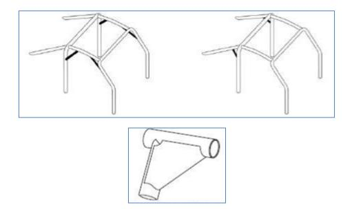
Reinforcement tubes must not be attached to the body shell.
