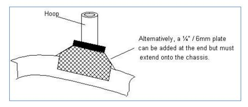
Main Hoop Design and Installation for Range Rover / Discovery and other Long Wheelbase Station Wagons
