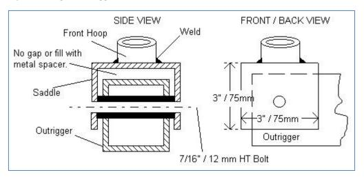
The hoop is welded to the saddle, and the saddle is attached to the outrigger with the high tensile outrigger /bulkhead bolt (which also secures the bulkhead)
