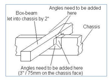
This method is stronger than reinforcing existing outriggers or adding fabricated ones. Spreader plates are not required where the roll-cage tube is welded on to 1/4" / 6mm wall thickness box material.
