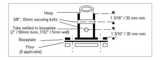
Above is a type of mounting enabling the roll-cage to be removed leaving only the socket in place in the vehicle.
