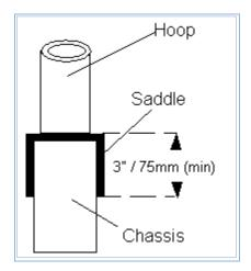
The Front hoop bulkhead assembly should be welded to fabricated outriggers made up of box channel 75 mm x 50 mm x 3 mm welded onto a base spreader plate of 6" by the depth of the chassis of 6mm. additionally a flat bar 6mm must be welded on the horizontal plane across the chassis. See diagrams below of suggested methods.
