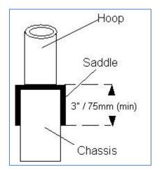
This shows the basic principle of a "U"-shaped channel welded over the chassis. There must be no gaps between the channel and the chassis.
