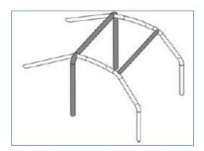
Tube ends should be correctly shaped to fit the bar they are joined to. Bend radius must be at least three times the tube diameter.
