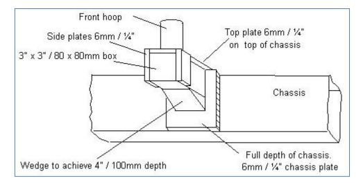
The drawing above shows how the 4" / 100mm depth at the chassis can be achieved. The wedge must be at least half the span of the outrigger.
