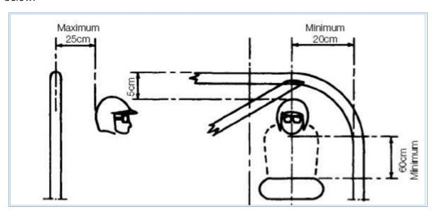
An effective roll over bar must be fitted of a height not less than 50 mm at its top edge above the helmet of the normally seated driver. It must be wider than the driver's shoulders at the height. Diagram of driver 20cm.
