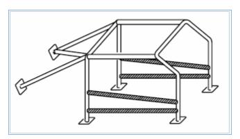
Vehicles with DOORS should have two crossed tubes welded from the front hoop to the rear hoop. (see diagram)
