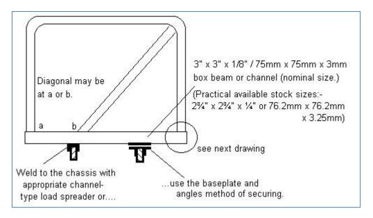
The design shown above is for use in Range Rover, Discovery and any other Long Wheelbase station- wagon vehicles. They give a more stable base due to the extra width of these vehicles and give back seat accessibility
