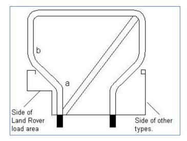
Above left shows the basic design. The less the amount of bend at points 'a' and 'b' will proportionately increase the strength of the bar. The bend at 'a' can effectively be reduced to a straight tube.
